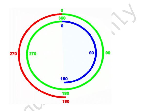
Blue 0 to 180 is the dot (flashing) PH over travel (Right 180 side of diagram) Red 0 to 180 is the dot(non flashing) PL over travel (Left 180 side of diagram)
