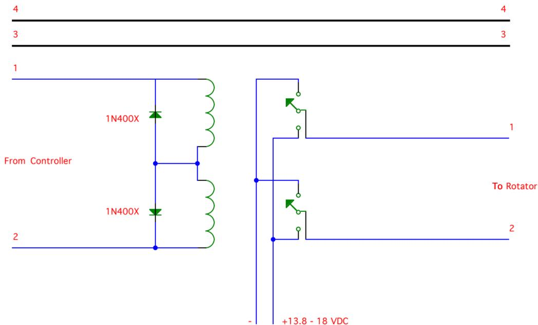
Relays chosen should be suitable for the proper coil voltage, as well as appropriate current carrying capacity of the contacts. A relay capable of 5 to 10 amps DC is adequate. The diodes are general-purpose 1 amp style such as the 1N400X series.
