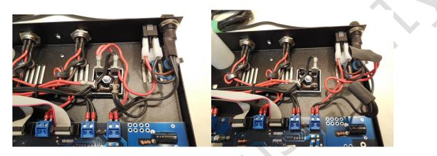
At this point you can apply power to the controller. The controller will operate normally except that when the direction buttons are pushed, the relays will click on and off but the rotator will not turn. If all is well remove power and continue.
